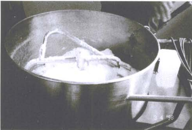
Figure 6 Modified cement mixer (Sakorn model)
